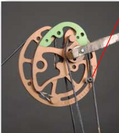
With the bow at full draw, as described above, a friend can note the position of the draw stop screw in relationship to the buss cable. The markings on the top cam are so you can have a reference point for the draw stop adjustment. **The adjustment should never be made while the bow is at full draw, as injury could occur.**
