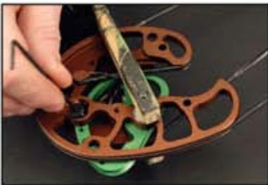
When adjusting Alpine one cams you have the option of adjusting draw length in 1/2 inch increments. To do this, simply move the adjusting screw from one mounting hole to the other. When doing this shift the rotating module to line up with the new hole location.
