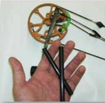
Included with your new Silverado Series bow, you will notice 2 - small 3/8" carbon rods. These rods are designed specifically for the purpose of loading or cocking the cam.
