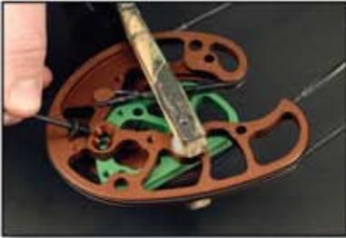
Start by removing the screw that is holding the draw module in place (the screw placement for your cam is pictured above).
